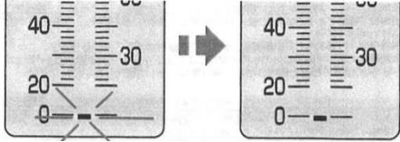
The diagram shows two states of a digital sphygmomanometer's LCD display. On the left, the display shows a scale from 0 to 40 with a dot flashing at the 0 mark, indicating 'Zero setting in progress'. An arrow points to the right, where the display shows the same scale with the dot lit up at the 0 mark, indicating 'Ready for measurement'.
